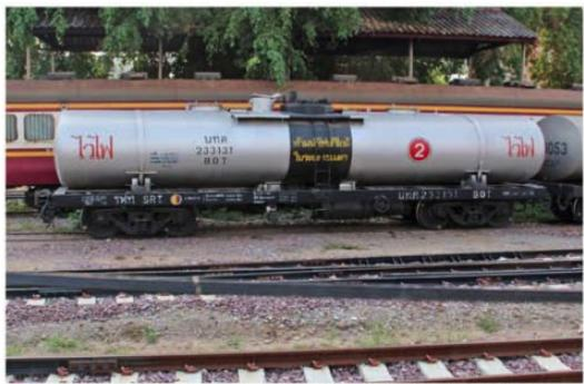
The major traffic to hear is oil transported in trains of these tank cars. They look squashed compared to those in the US. The shape makes sense: the center of gravity is significantly lower making the cars more stable on the narrow gauge tracks.
